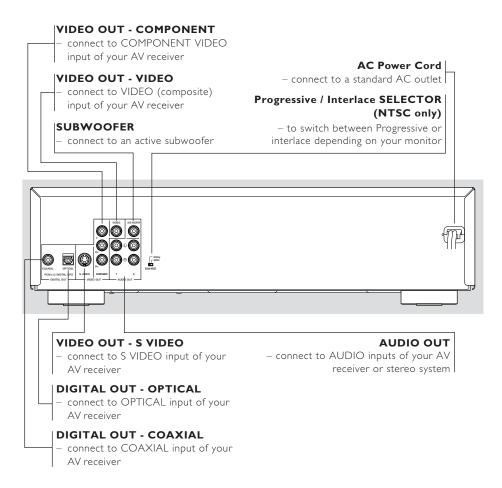
Caution: Do not touch the inner pins of the jacks on the rear panel. Electrostatic discharge may cause permanent damage to the player.
